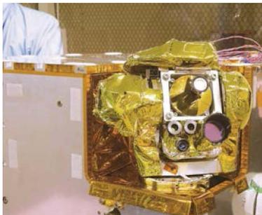
Fig. 3. NICT’s SOTA flight model onboard SOCRATES.
